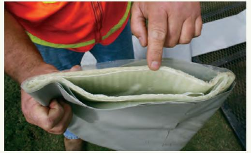
The CIPP method is an effective and non-invasive form of sewer line rehabilitation.
